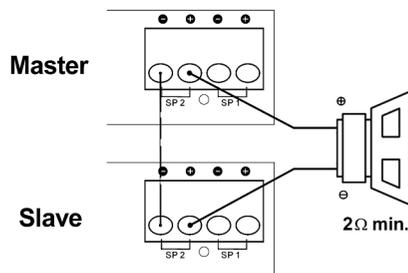
**CAUTION:** Two ECS 1200.1 amplifiers that are strapped together are not recommended for impedance loads below 2Ohms.
