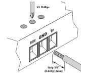
5. Prepare the BLACK wire (Ground cable) for attachment to the amplifier by stripping 5/8" of insulation from the end of the wire. Insert the bare wire into the GROUND terminal and tighten the set screw to secure the cable in place. Prepare the chassis ground by scraping any paint from the metal surface and thoroughly clean the area of all dirt and grease. Strip the other end of the wire and attach a ring connector. Fasten the cable to the chassis using a non-anodized screw and a star washer.
