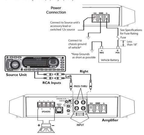
NOTE: Outputs are wired in parallel internally.
