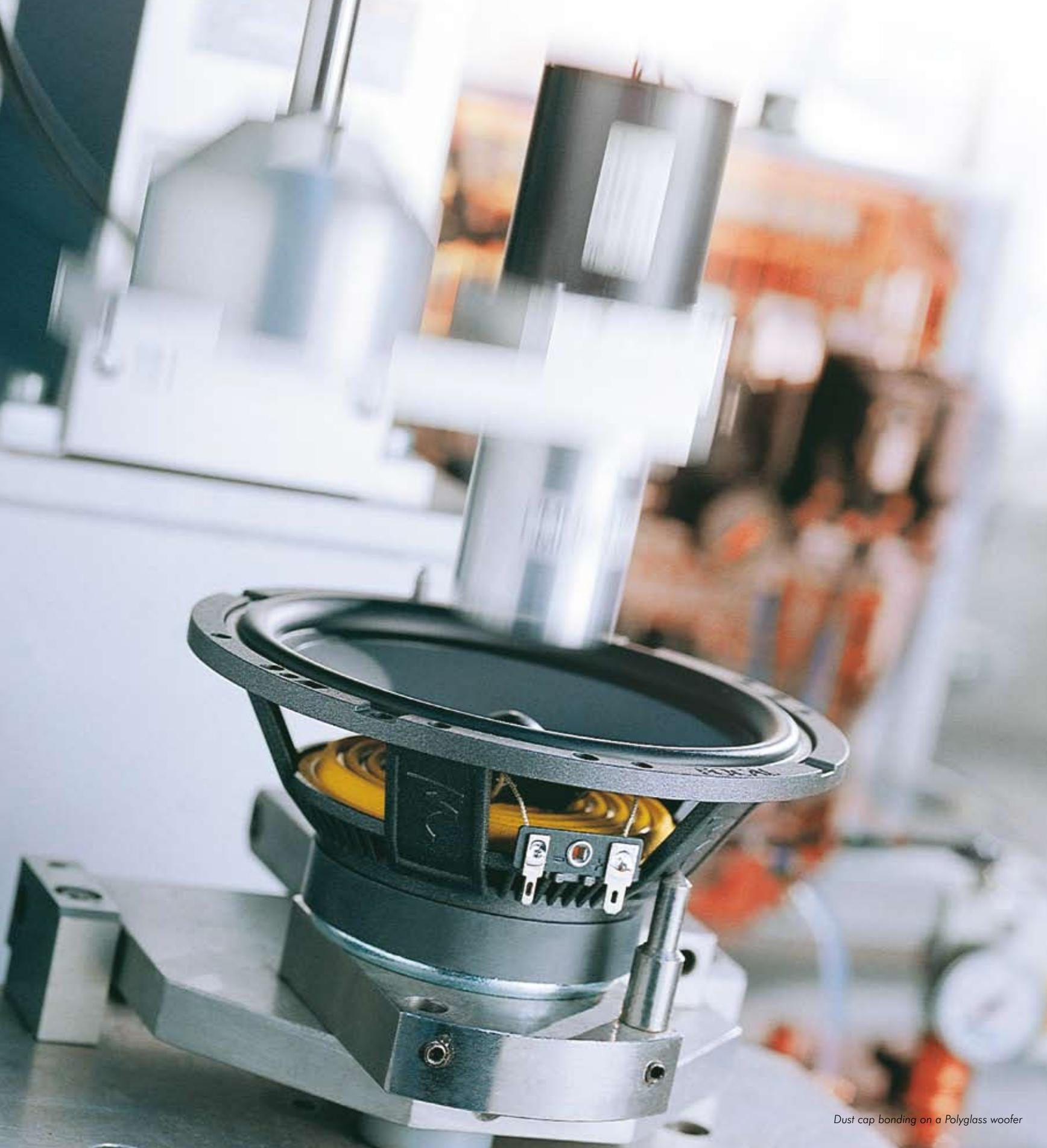
*Dust cap bonding on a Polyglass woofer*
