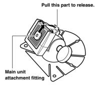
2 Loosen the main unit attachment fitting with a coin etc., slide it into the track on the rear of the main unit and temporarily fasten it. Then fix it to the stand.
