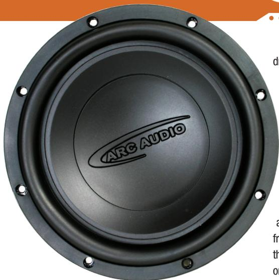
for a little less efficiency but more low frequency output. In terms of a vented application, Arc Audio suggests a 0.6 cubic foot enclosure with a 2-inch ID vent with a length of 12 inches. This tunes the enclosure to 34Hz and was the one I decided to go with. Long-time friend Mark Feeney at Sell Thru Displays custom built the enclosure for me and I took care of the speaker cutout and vent back at the test lab.
