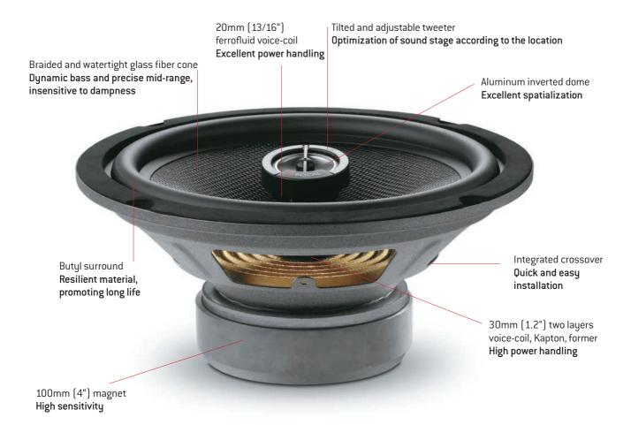
200mm (8") woofer, 30mm (1.2") voice-coil, 100mm (4") magnet Adjustable aluminum inverted dome tweeter Integrated crossover (5.2kHz) Max. power: 160W Nom. power: 80W Sensitivity (2.8V/1m): 93dB Frequency response: 50Hz – 20kHz
