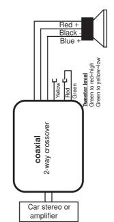
On the cable filter box without screw terminals the level select is made on the outside by connecting the green cable to either the red or yellow one coming out from the box.
